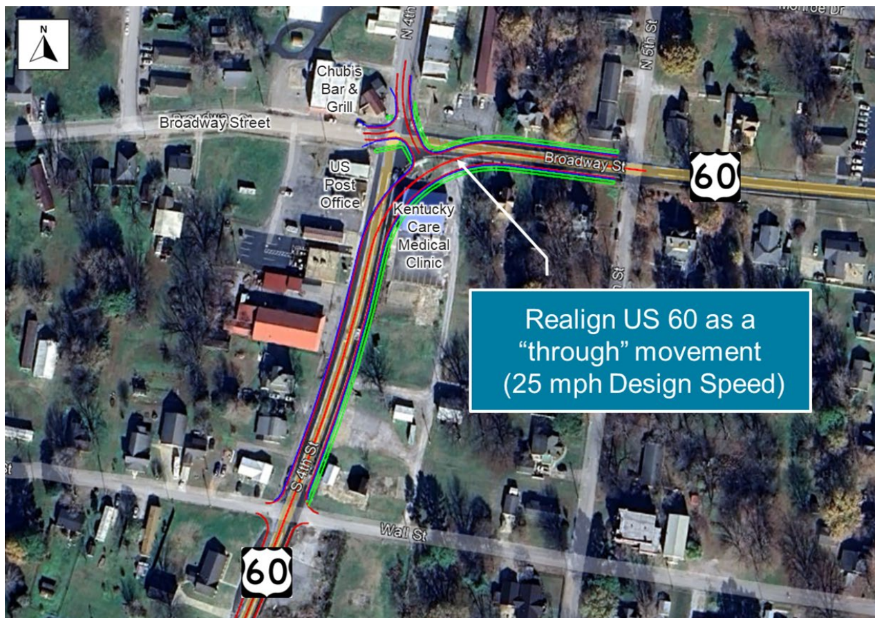
Figure 24: US 60 at Broadway Street in Barlow - Realignment
